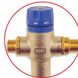
**Thermostatic mixing valve** – this device costs more than a tempering valve but can be set to deliver hot water at 50°C or below throughout the home. It's able to be serviced over time, and does not have a limited life.
